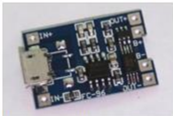
Figure-2 (b): Battery Charger
